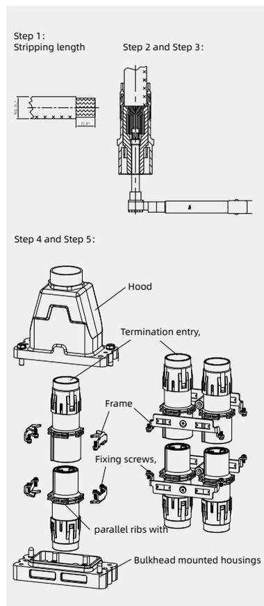
1) See P00-30-00-31 for the structural characteristics and description of Axial screw terminal.
